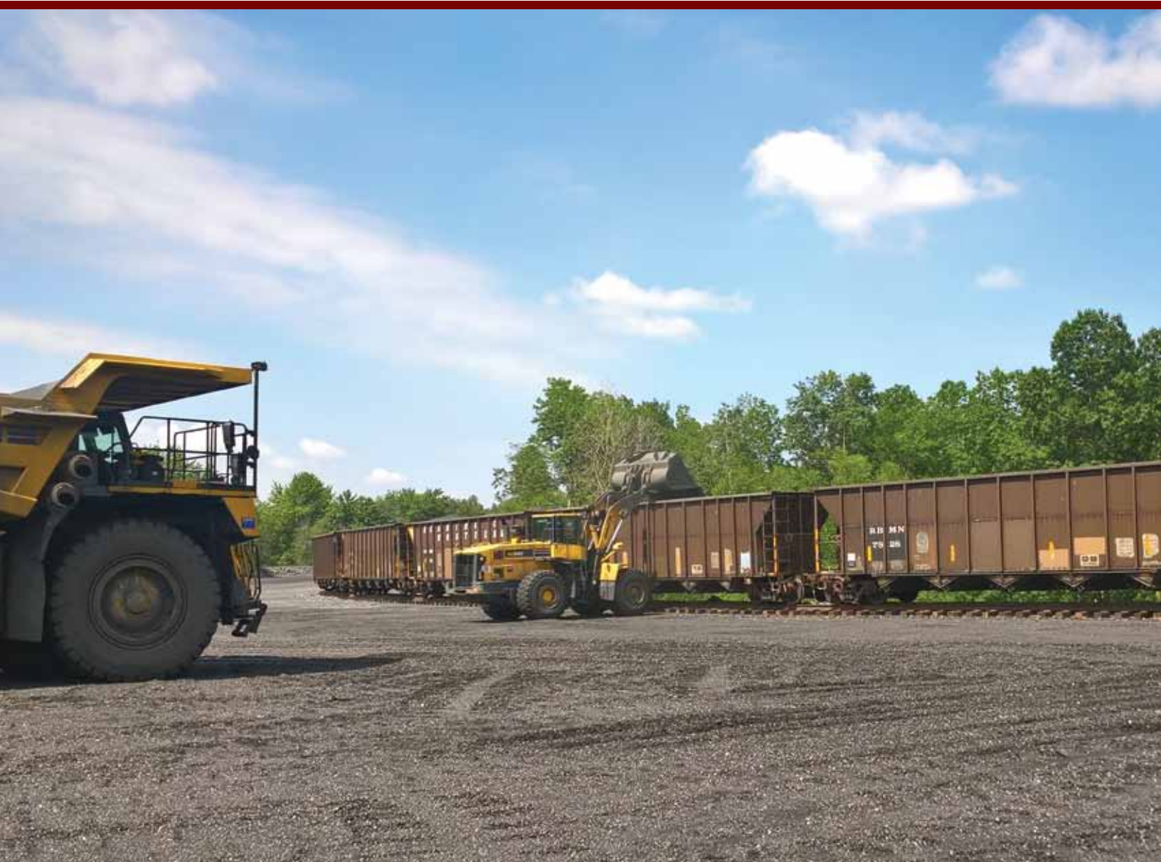
Rail cars are being loaded while a haul truck delivers more material to the load out.
