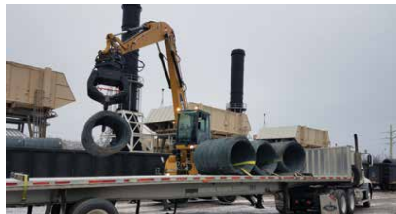
Loading steel coils onto a Reading Railroad Transfer truck at the West Hazleton Transload.
