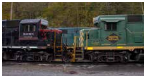
No. 2012, one of three once-high-nose GP38-2s purchased from Norfolk Southern, shows off its cut-down nose for better visibility.
