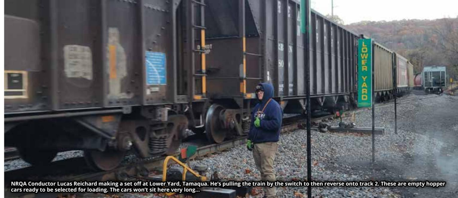
NRQA Conductor Lucas Reichard making a set off at Lower Yard, Tamaqua. He's pulling the train by the switch to then reverse onto track 2. These are empty hopper cars ready to be selected for loading. The cars won't sit here very long...
