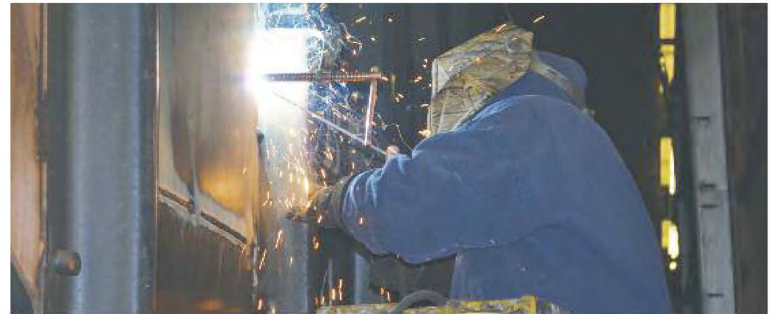
Tom Stemko welding a patch on an aluminum coal car.
